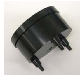
Photograph No. 4 Transmitter Puck – Rear
